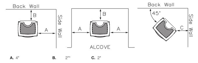
Heater should not be installed directly on carpeting.
