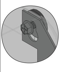
Tabs located on either side of ice bucket must engage notches in side shelf.
