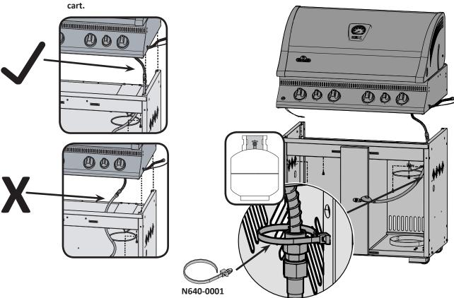
Clip hose to side panel using hose retainer clip supplied.
