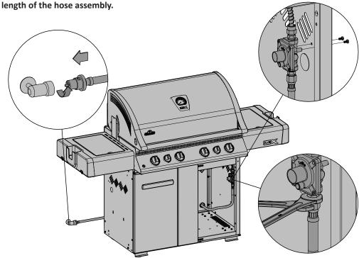
This unit includes an internal regulator which stabilizes the gas pressure and improves grill performance. This regulator cannot be adjusted. There is a pressure tap located on the side of the regulator. It can be used by a qualified service person when servicing the grill to determine if the regulator is functioning properly. The screw within the pressure tap must always be kept tight, except when performing a pressure test on the regulator (qualified service personnel only).
