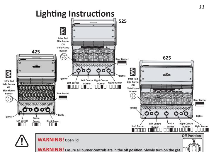
**WARNING!** Ensure all burner controls are in the off position. Slowly turn on the gas supply valve.
