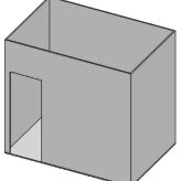
Within a partial enclosure that includes an overhead cover and no more than two sidewalls. These sidewalls may be parallel, as in a breezeway, or at right angles to each other.
