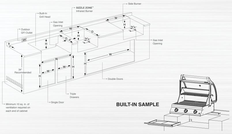
Please use manual to properly assemble your built-in grill. Refer to the main manual for operating, cleaning, and maintenance instructions. This grill is designed for non-combustible enclosures only, and must be installed and serviced by a qualified installer to local codes. Drawings for reference only. Minimum 6" clearance required between grill and other appliance. Specifications subject to change without notice. \* Additional clearance may be required for openings. See owners manual
